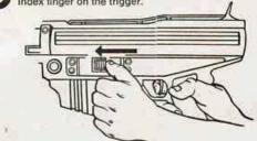
Load racer and cartridge into the loading chamber, nose first, pushing them all the way forward and into position.
