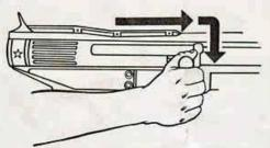
To remove the cartridge, rais: the bolt of the rifle and pull it towards the rear of the rifle This will automatically eject the cartridge. Reload your ram and you're set to go again.
